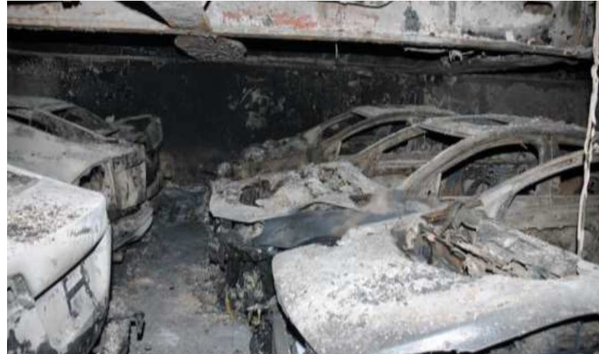
Figure 7: Completely burnt out vehicles on deck 3 B
